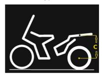
d) Then take the same measurements with the rider and equipment on the motorcycle. It is important that the rider is balancing on the correct riding posture and repeat the measuring procedure one more time.
