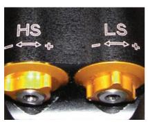
If the shock absorber speed is low, adjust the LS knob, for example if the shock movement is initially too hard or too soft to provide enough comfort (more information in chapter "Which adjuster to change").
