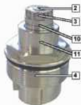
Fork cap with reversed preload
